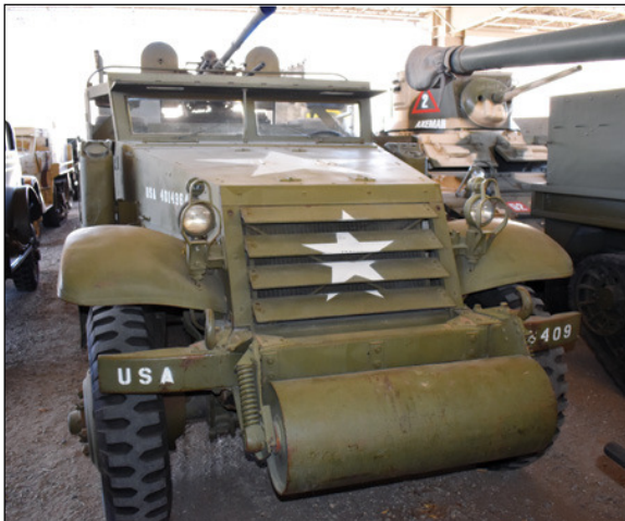
WWII era halftrack - tires up front, tank track in the rear.
