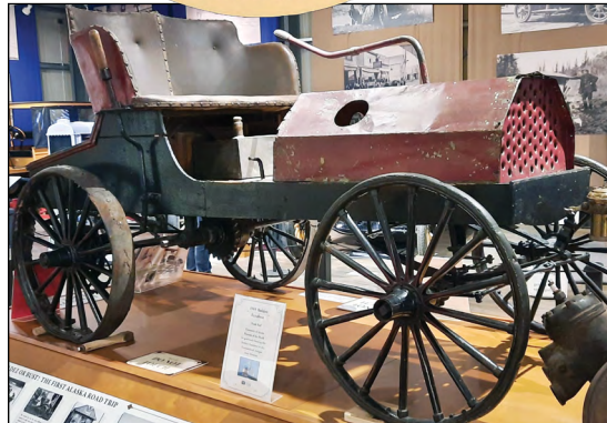
The vehicle Alaskan Bobby Sheldon built in 1905 from buggy wheels, a marine engine and two bar stools. He had never seen an automobile in person.
