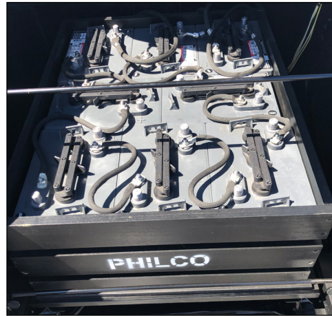
The Milburn Electric featured a rapid-exchange system for installing fresh batteries.
