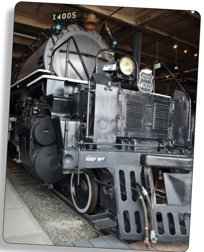
The imposing Union Pacific "Big Boy" was the largest locomotive ever built at 132 feet long and weighing 1.2 million pounds.
