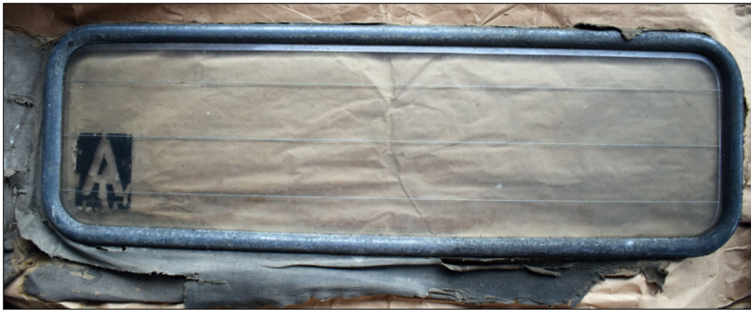
The original rear window for my 1928 Stutz Model BB cabriolet featured an early form of safety glass with metal wires running through the glass.
