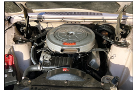
The 390 cubic inch V8 engine produces 300 horsepower.
