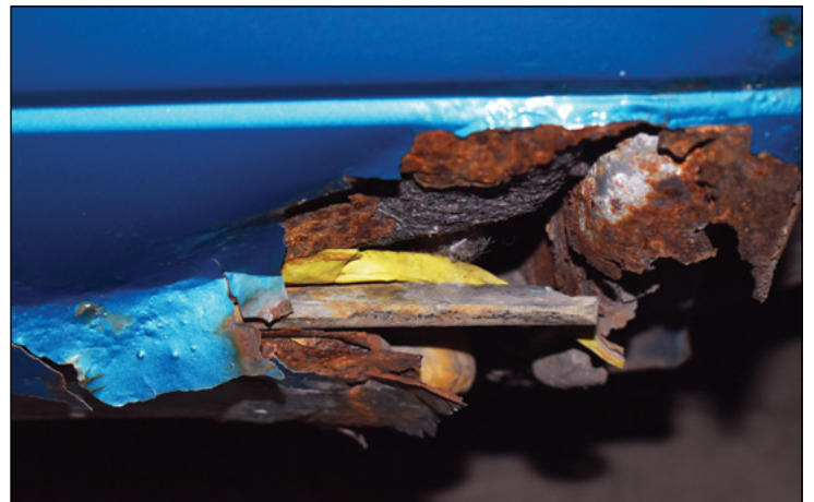
Severe rust out developed on both rocker panels after driving the Thunderbird for several years in all kinds of weather.
