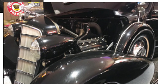
1935 Cadillac V8 engine with the Detroit Lubricator Carburetor
