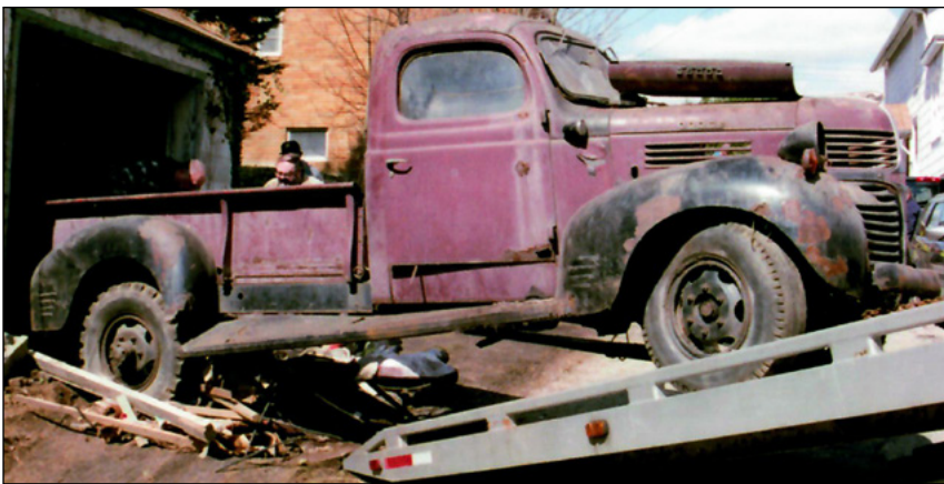
The old tires held air but the brakes were rusted to the drums thus preventing the rotation of the wheels. Note the debris it dragged towards the ramp.
