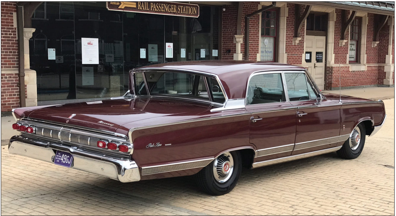
The 1964 Mercury Parklane is 18 feet long and features the unique “Breezeway” roof design. Tilted inward, the back window is divided into three sections. The middle section can be lowered to allow fresh air to flow through the passenger compartment.
