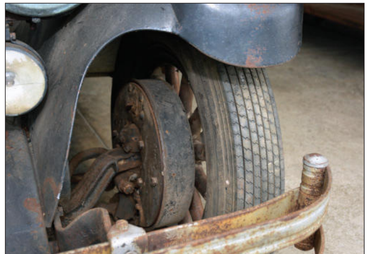
Progressive Willys installed four-wheel brakes on the Knight in 1927.
