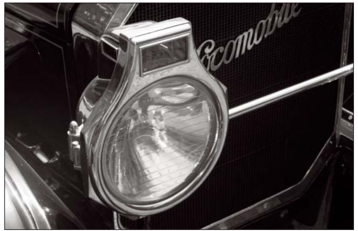
The distinctive shape of the nickel-plated headlight buckets was characteristic of Locomobile for years. The projections above the headlights are the parking lights, innovatively visible from the front and the sides.
